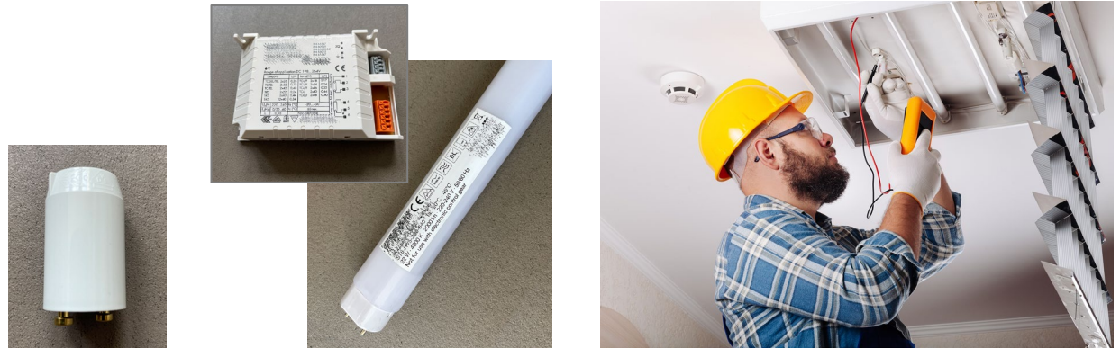
Figure 9 | “LED starter” – electrical bridge – to replace the starter for luminaires with electromagnetic ballasts (LLB) with “retrofit lamps” (left), conversion kit to bypass the previous ballast – rewiring – (middle) [© Fraunhofer IBP] and conversion of the luminaire on the ceiling (right). [© Billion Photos / Shutterstock]
